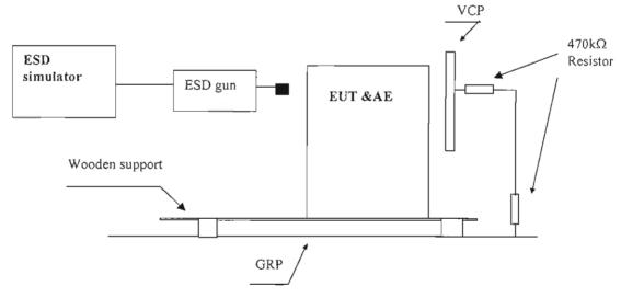
Note: VCP means <u>Vertical Coupling Plane</u> GRP means <u>Ground Reference Plane</u>
